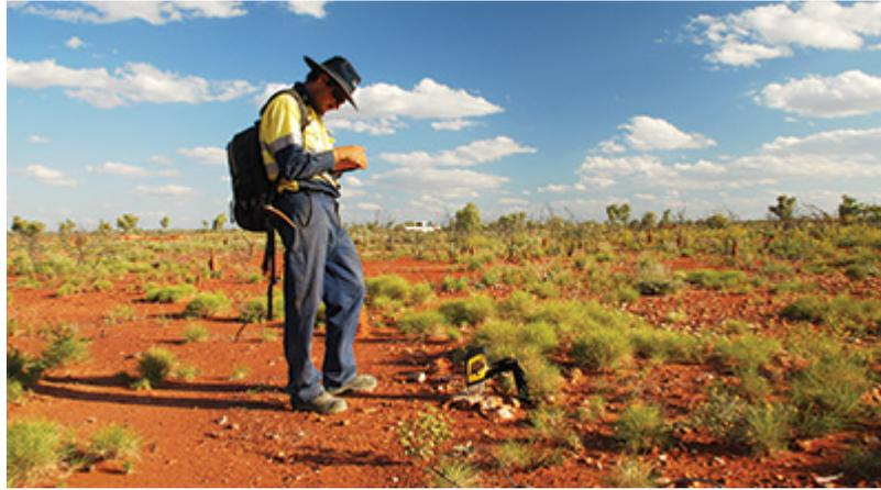
*Figure 2. Example of a hand-held portable X-ray analyser (pXRF) used in the field in for a previous project worked by the exploration staff engaged for EL006408.*
